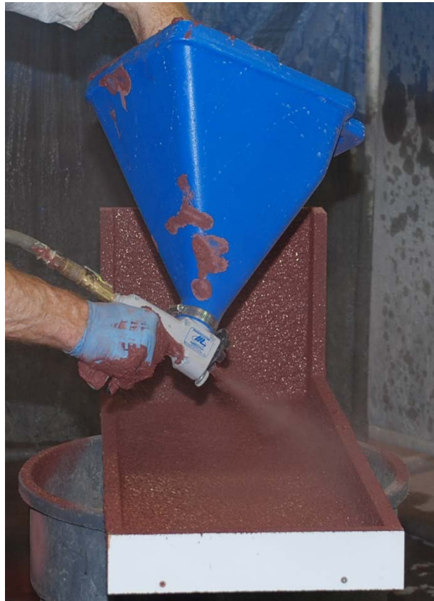
Figure 7:Spraying the face coat
