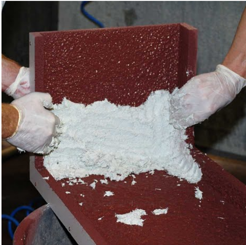
Figure 8: Hand packing backer on upright
