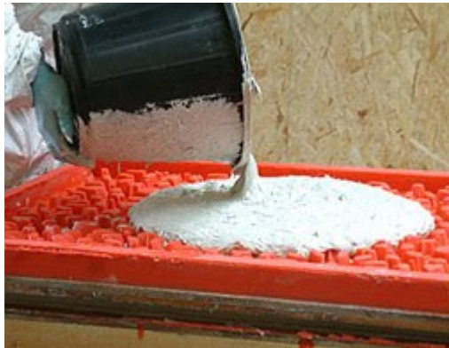
Figure 6: Premix Zoho Stone's GFRC pouring into a mold
